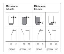
Diagram showing function of the **electronic** switch and LEDs
