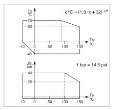
Top graph: Limit values for ambient temperature  $T_U$  at housing are dependent on the operating temperature  $T_B$  in the tank.
